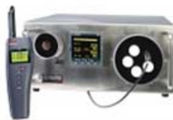
Humidity generator (ROTRONIC- HYGROGEN-2)
