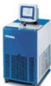
Liquid bath for temperature (WIKA-CTB 9400)
