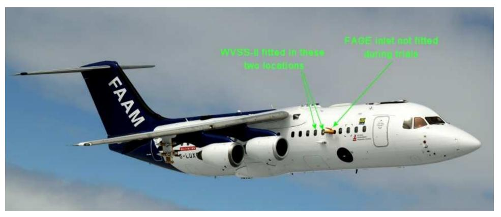
Two WVSS-II units on separate window plates
