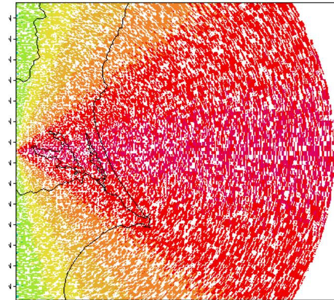
Simulated uniform wind field with speeds of 50 m/s.
