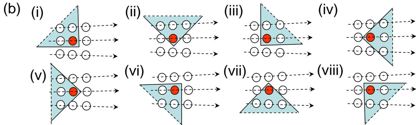
A spatial linear approximation is applied using the velocity,  $v'_{can}$ , to derive the approximation of the unfolded Doppler velocity. The approximated value that has the smallest sigma in the available all sampling patterns is set to the reference data of the target bin.
