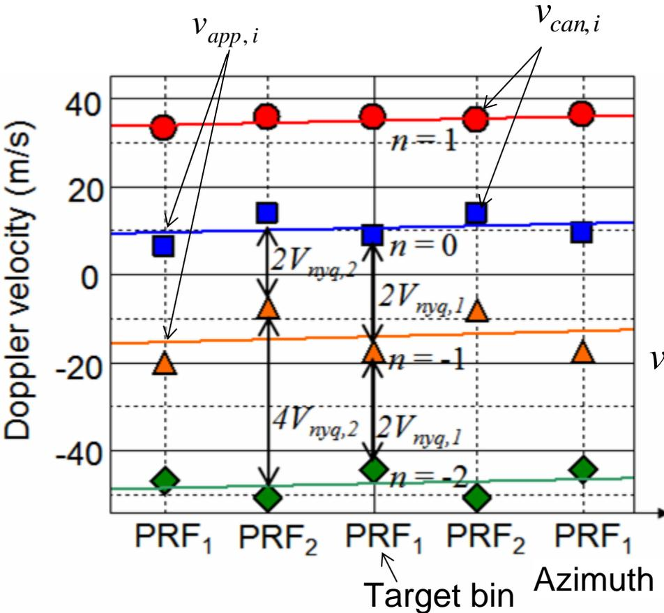
A slice along the azimuthal direction of the candidate and approximated Doppler velocity fields of each possible unfolded Doppler velocity.
