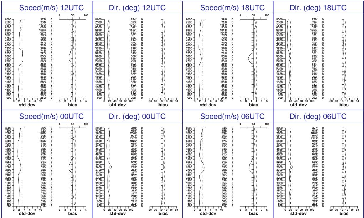
Figure 5. MeteoFrance monitoring results for the Lindenberg 482 MHz RWP for March 2003. The effects of WT clutter are clearly visible at heights between 2.5 and 3.5 km.
