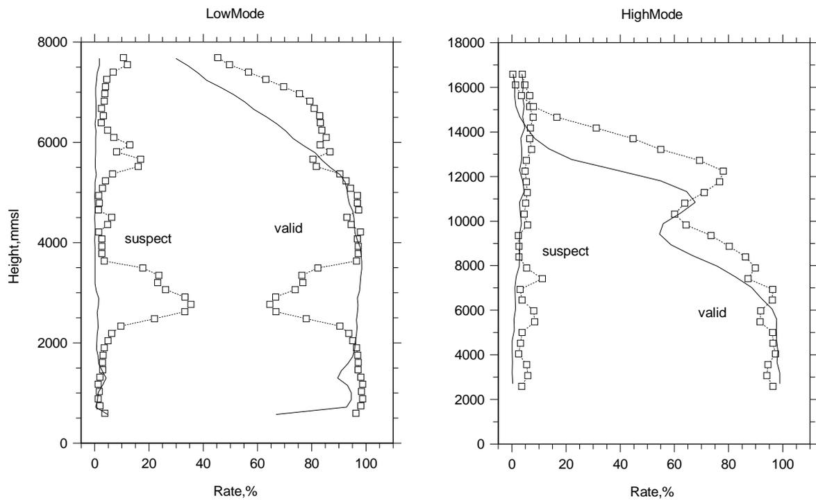
**Figure 4.** Rate of valid and suspect wind data measured with 482 MHz wind profiler as function of height in March 2002 (solid line, undisturbed situation) and in March 2003 (squares, disturbed situation)
