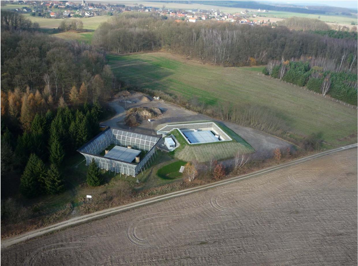
**Figure 1.** Old and new 482 MHz RWP at Lindenberg. While the first installation was surrounded by a metallic clutter fence, the new radar is shielded by a berm.
