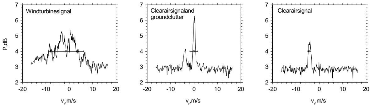
Figure 6. Power spectra illustrating a wind turbine, a ground clutter and a clear air signal
