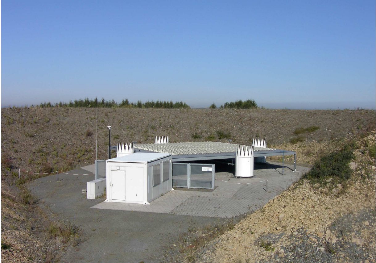
Figure 3. Photograph of the 482 MHz RWP installation of DWD at Bayreuth (Oschenberg), showing the antenna array platform surrounded by four acoustic sources for RASS and the shelter containing the radar electronics.
