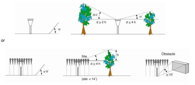
• Flat, horizontal land, surrounded by an open area, slope less than 1/3 (19°). For a raingauge artificially protected against wind, the instrument does not necessarily need to be protected by obstacles of uniform height. In this case, any other obstacles must be situated at a distance of at least 4 times their height.
