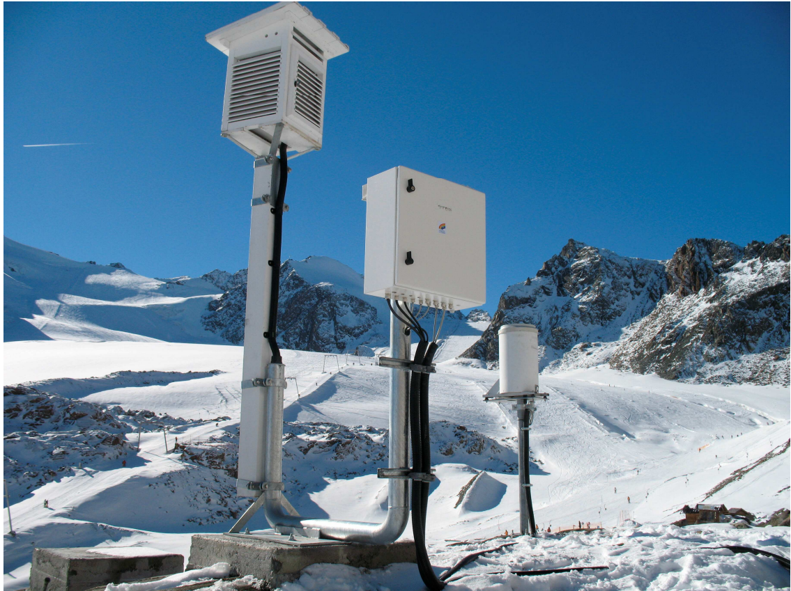
Fig. 13.: TAWES Station Pitztal Glacier - Sensor Station A in a High Alpine Environment
