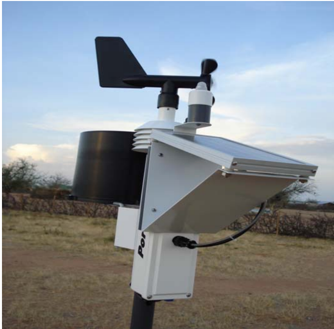
This AWS was installed by an NGO at a remote place in Kenya. All sensors are 3metres above the ground.
