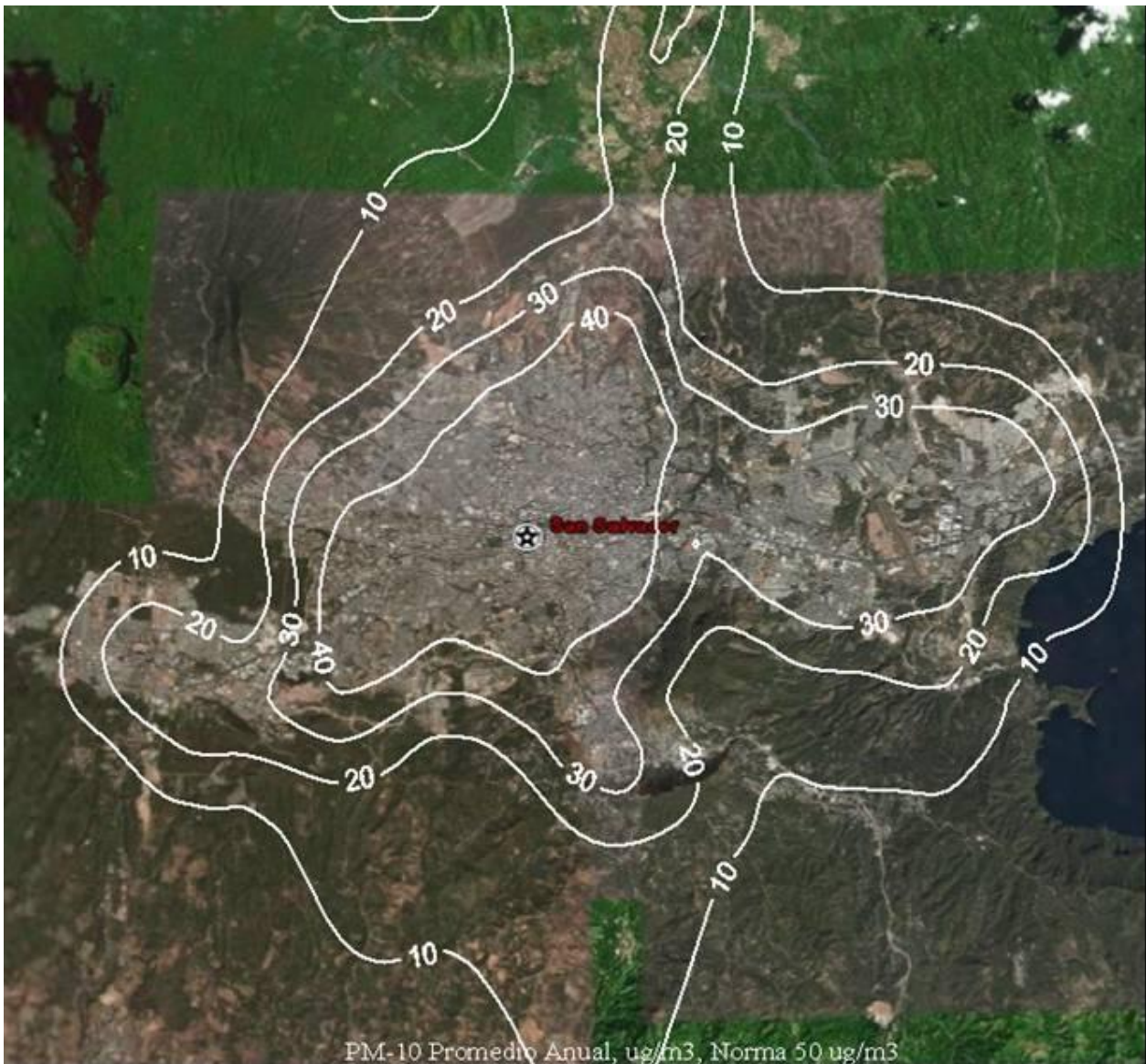
Aerial Photography of AMSS showing a map of Isolina model pollutant dispersion ISC3 with the annual average PM-10 in ug/m3 for comparing with the Standard Reference 50 ug/m3 per year.
