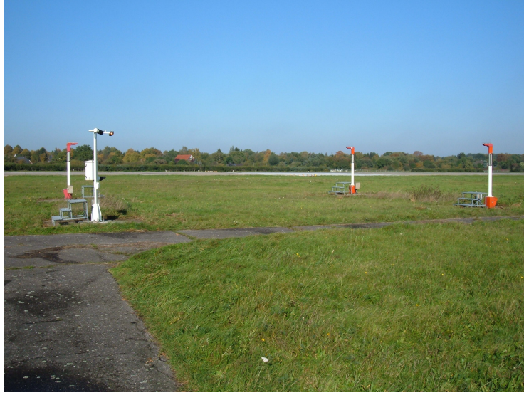
Fig. 2: Skopograph II transmissometers and DF20+A forward scatter sensor at Hamburg airport.
