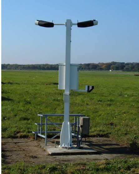
Fig. 1: DF20+A with ambient light sensor (LU320).
