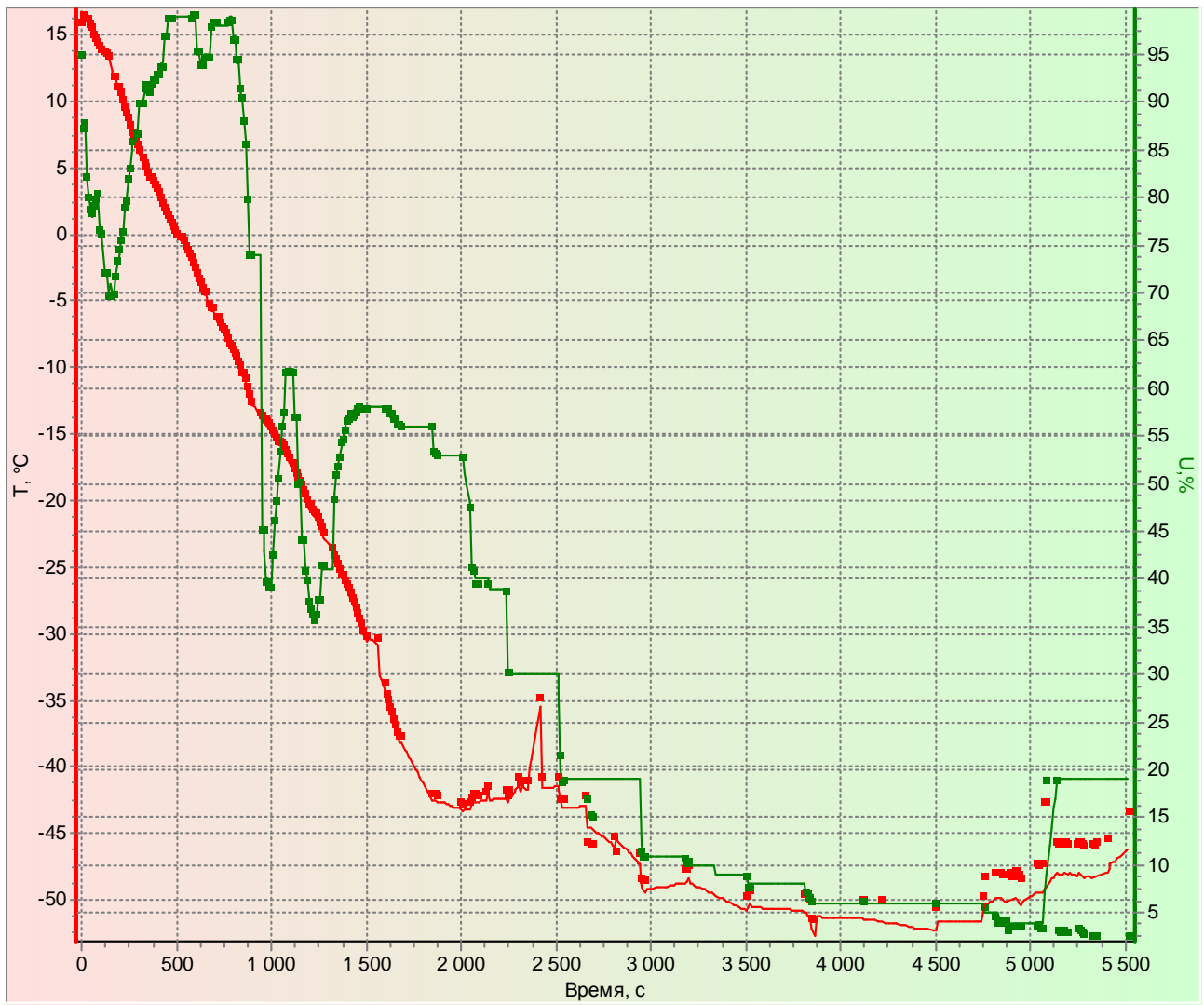
Figure 19. Primary (points) and edited 10 (lines) temperature [°C] and humidity [%RH] – massive data loss and outliers.
