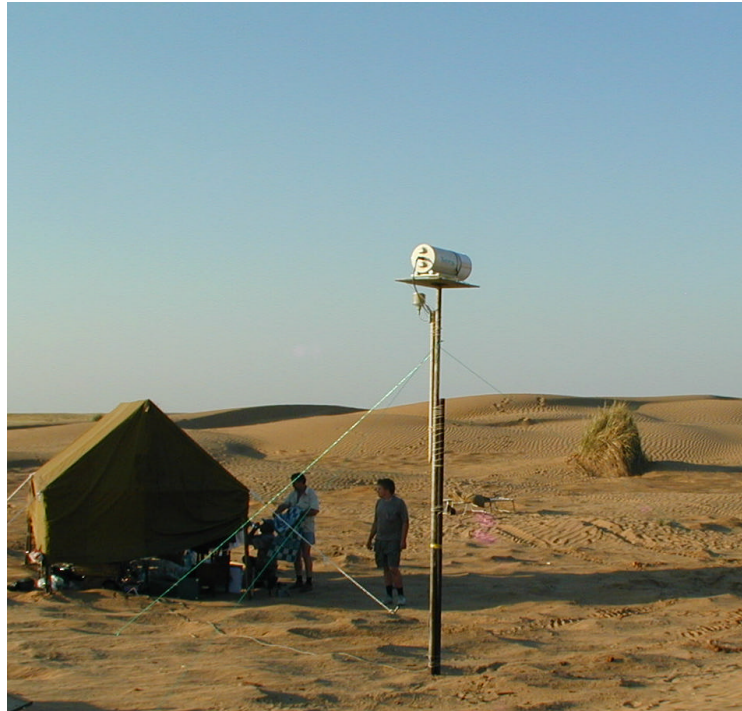
Fig.2. Microwave temperature profiler MTP5 at arid region.
