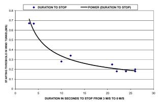
A defined accepted starting threshold allows to provide a criterion duration. For example, for a given type of sensor used in Météo-France network, this duration must be greater than 22~s for anemometer, and 10~s for vane, for a starting threshold of 0.5~m/s.
