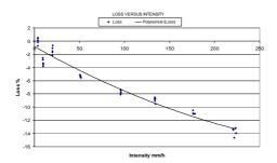
The important quality for rain gauge is a good repeatability of the buckets' response, providing a stable error, easy to set when adjusting the rain gauge. A better repeatability is obtained using a large bucket capacity (20 g) rather than a small one. It allows a reduction of wetting losses, to enhance repeatability by enlarging cone nozzle.
