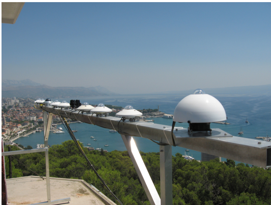
Figure 2. Pyranometers on the mounting platform at the roof of Meteorological observatory Split-Marjan
