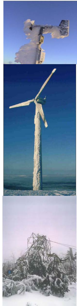
Pictures 1-3: Striking views of frozen meteorological instrument (top), wind turbine covered with ice (middle) and damaged power line (bottom).
