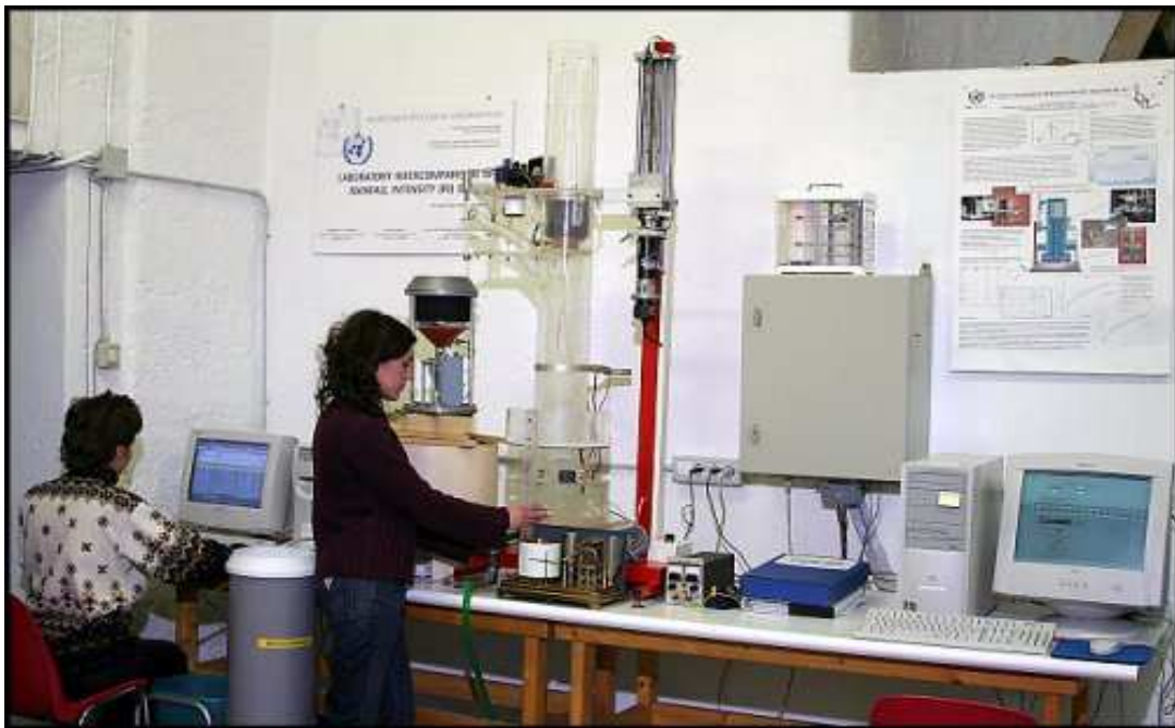
Fig. 1: The Qualification Module for Rain Intensity Measurement Instruments developed at the University of Genova.
