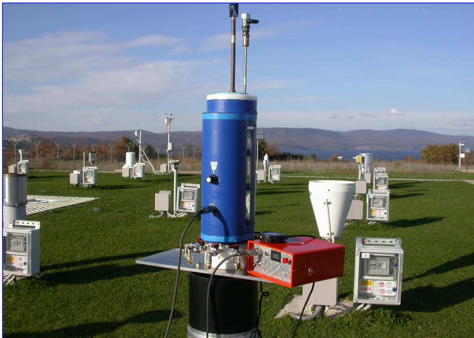
Fig. 8: The portable device for field calibration of catching type gauges in use during the WMO Field Intercomparison of RI gauges.
