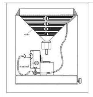
Heater power : 24 VAC, 60 W at the base Air temperature : Between +3 – (-5) °C
