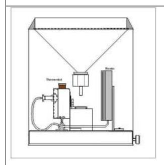
Heater power : 24 VAC, 43 W at the base : Between +3 – (-5) °C
