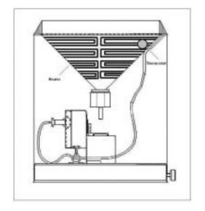
At the situation heater and thermostat are connected to the same surface, the surface temperature of water collecting cone becomes between +4 - +12 °C.
