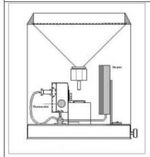
Heater power : 24 VAC, 43 W at the base Air temperature : Between +3 – (-5) °C
