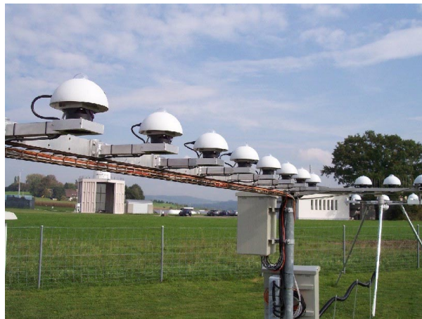
Figure 1, Biometers measuring concurrently the erythemal UV irradiance for a calibration check period at the BSRN Payerne (Switzerland) station of MeteoSwiss.
