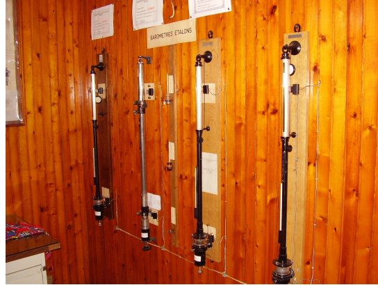
Fig 5.2 Pressure Room containing mercury standard barometer reference and working standard barometers (type FORTIN)
