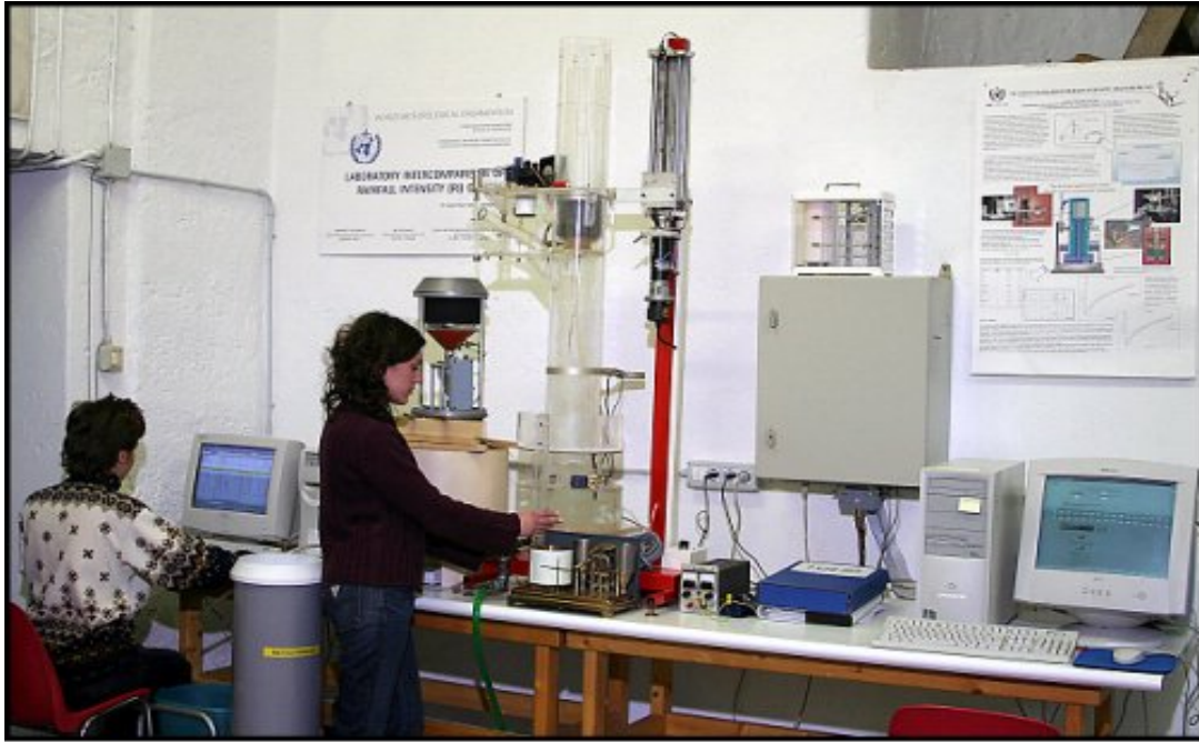
Fig 1: The Qualification Module for Rain Intensity Measurement Instruments developed at DIAM.
