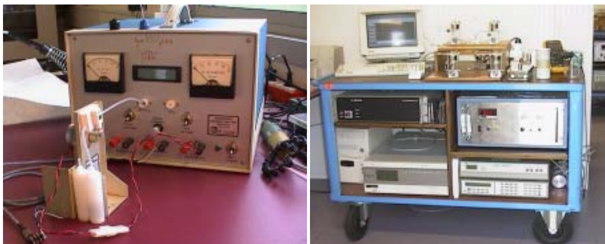
Figure 2: Left: Standard units for ECC ozonesonde preparation prior to the flight. Right: Laboratory equipment developed at MeteoSwiss for the preparation and testing of ozonesonde.
