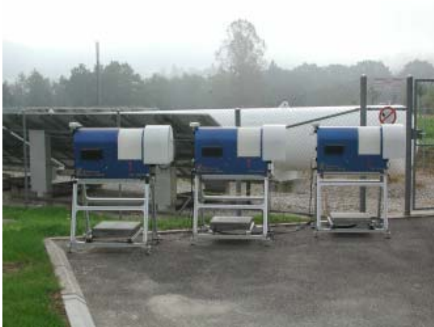
Figure 1. The three microwave radiometers installed at the aerological station of Payerne, Switzerland.
