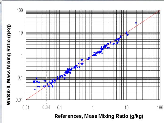
WVSS-II will give valuable results for mixing ratios above 0.04 g/kg. For typical mid-latitude humidity profiles the useful vertical measuring range is about
