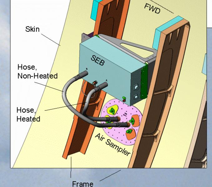
The sensor system is installed at the nose section on the right hand side of the aircraft below passenger door #1.
