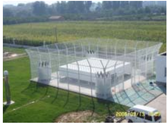
Fig. 4: CFL-08 Wind Profiler Radar with RASS
