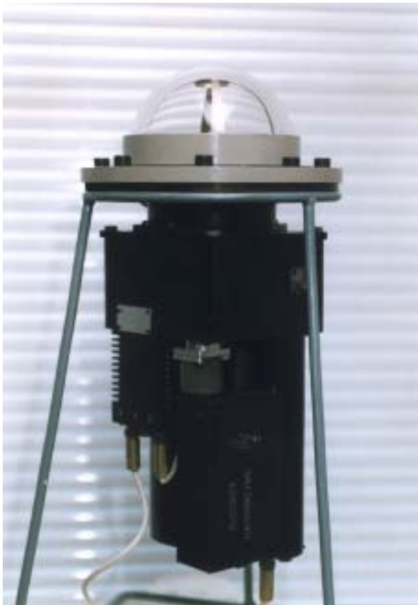
Figure 9. Spectral module of ultraviolet spectroradiometer PION-UV
