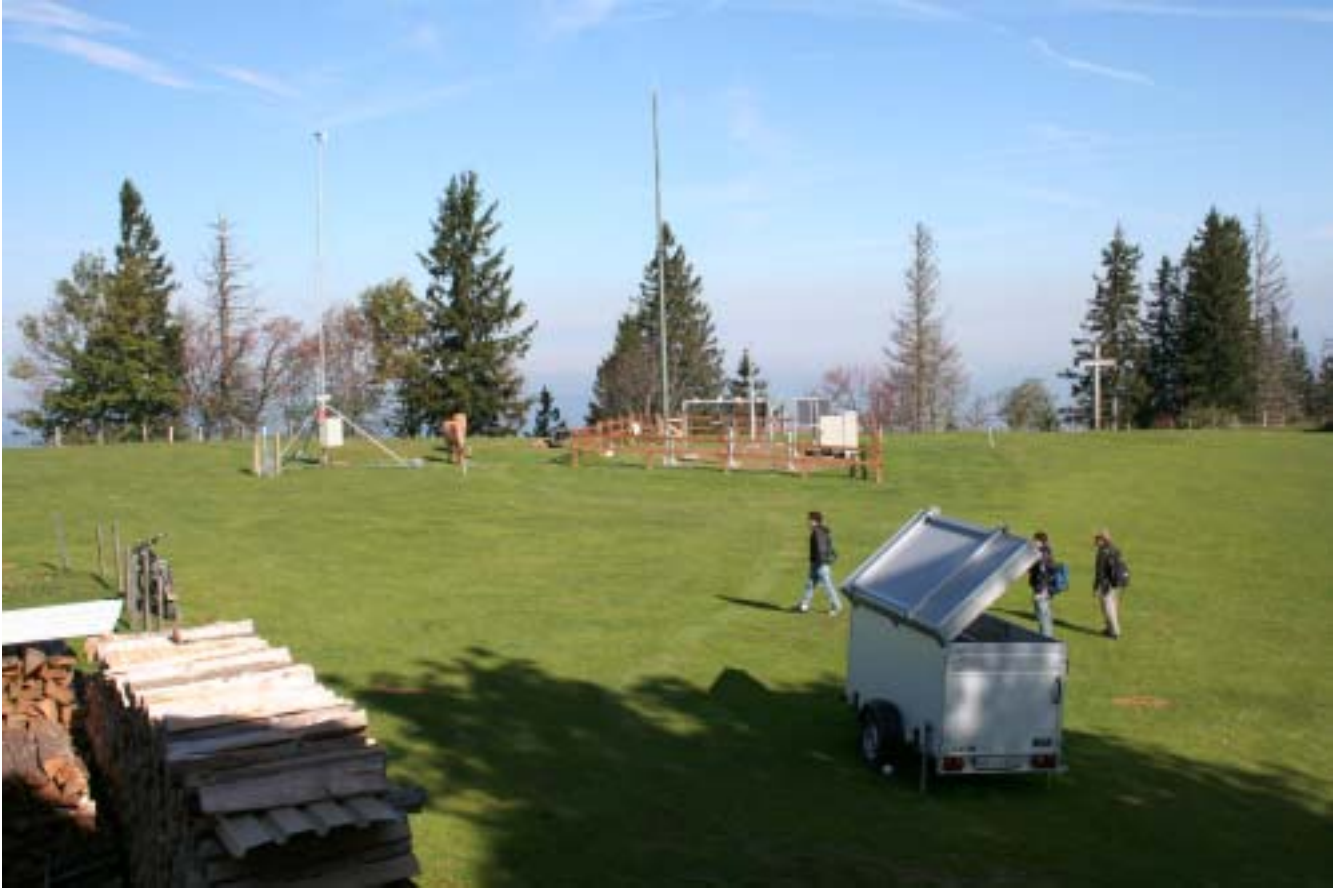
Picture 2: View of the mobile station installed nearby the SwissMetNet station at the Napf Mountain during construction in autumn 2006. The dedicated trailer (which can be transported by helicopter) may be seen at the bottom of the picture.
