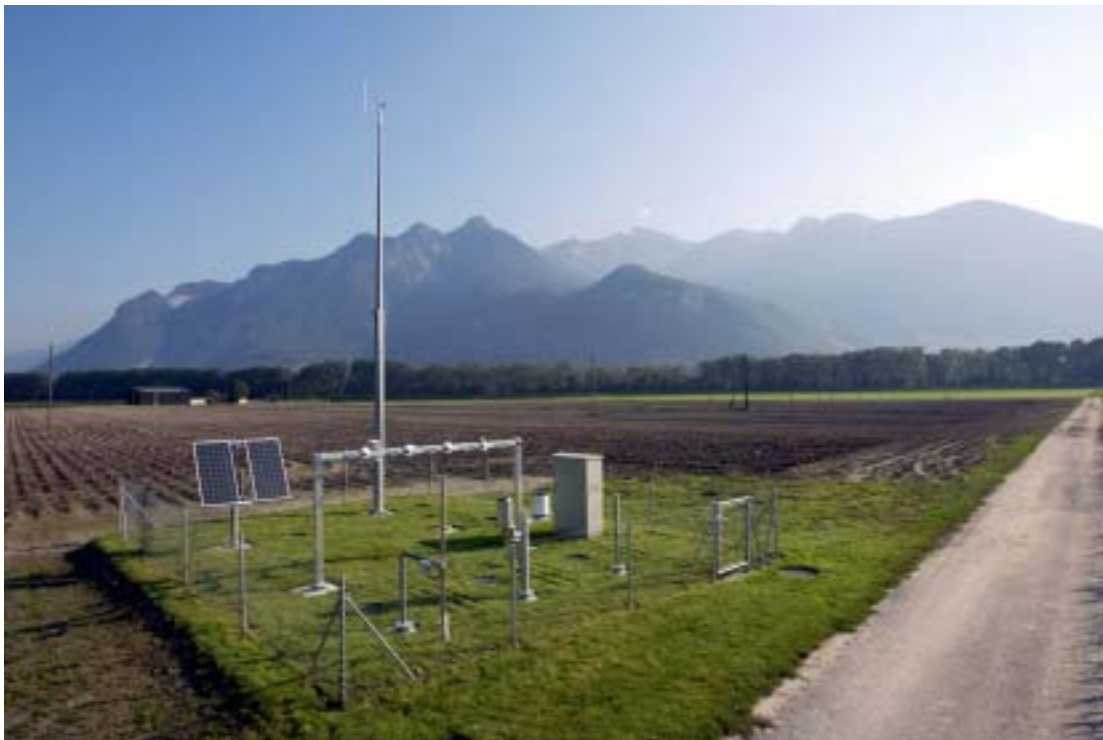
Picture 1: View of the model Westa B SwissMetNet station located at Aigle, VS, Switzerland, representing a complete configuration, but without snow height measurements.
