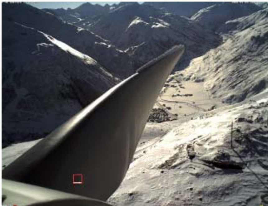
Picture 2: Icing at the blade of the operational E-40 wind turbine recorded automatically by a webcam mounted at the nacelle. The meteorological test station may be spotted on the right side of the picture nearby the 2 wind masts.
