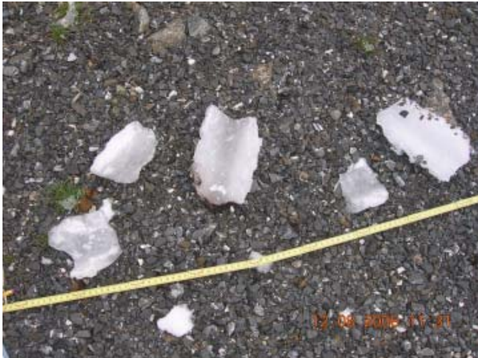
Picture 3: Ice throw of the E-40 wind turbine.
