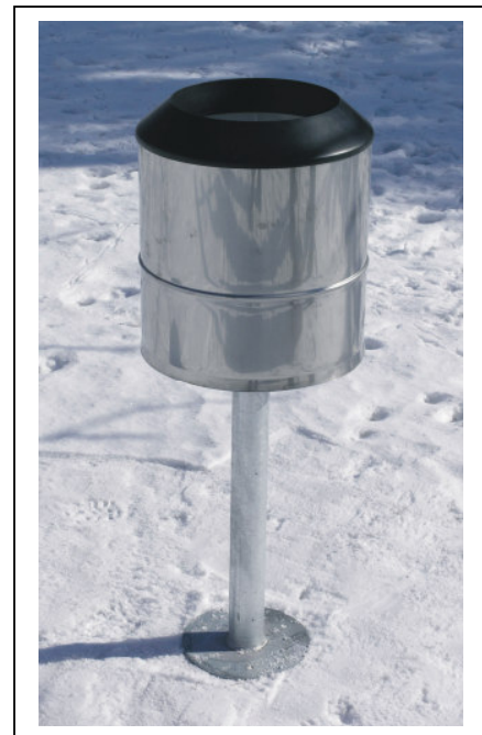
Fig. 1 Self correcting weighing sensor TRwS500
