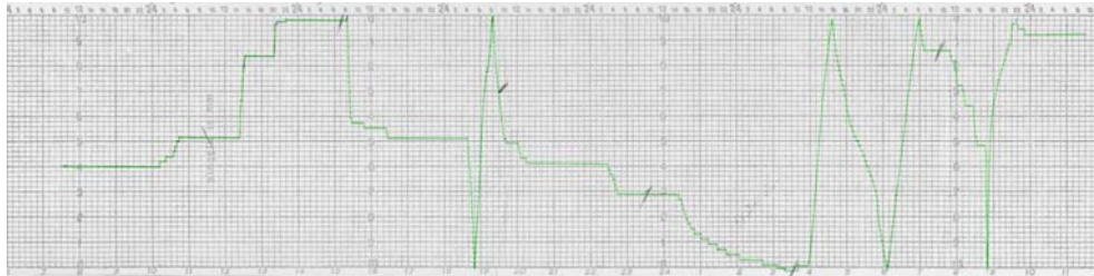
The track detected by the software is superimposed in green on the original rectified image
