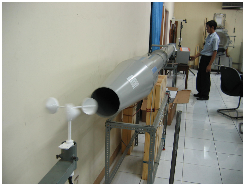
Figure 6. Wind Speed Sensor Calibration of AWS MGA-05 at Meteorological and Geophysical Agency
