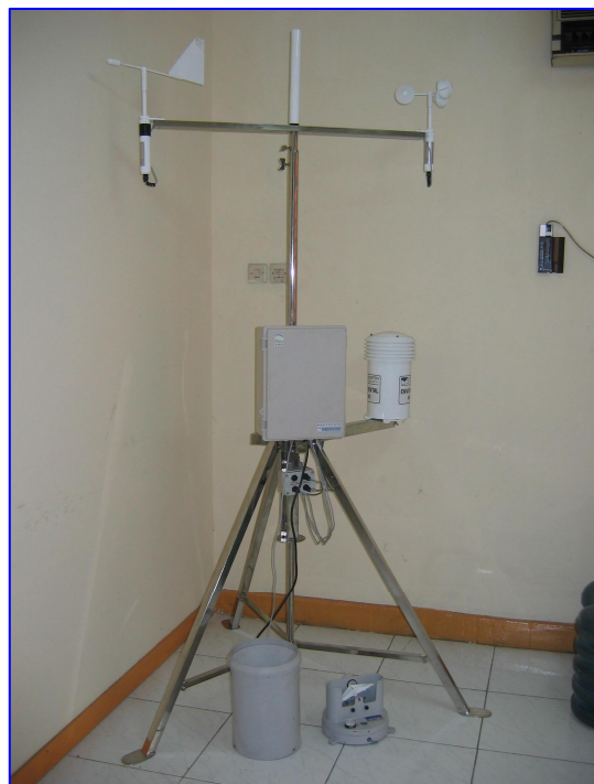
Figure 5. Sensor and the Data Logger System of the AWS MGA-05
