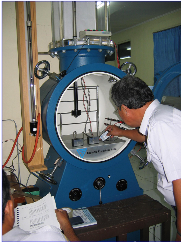
Figure 5. Pressure Sensor Calibration of AWS MGA-05 at Meteorological and Geophysical Agency
