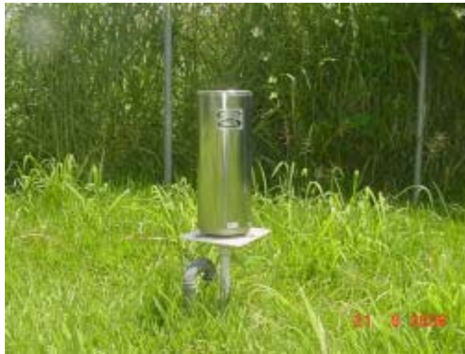
Typical Rain Gage
