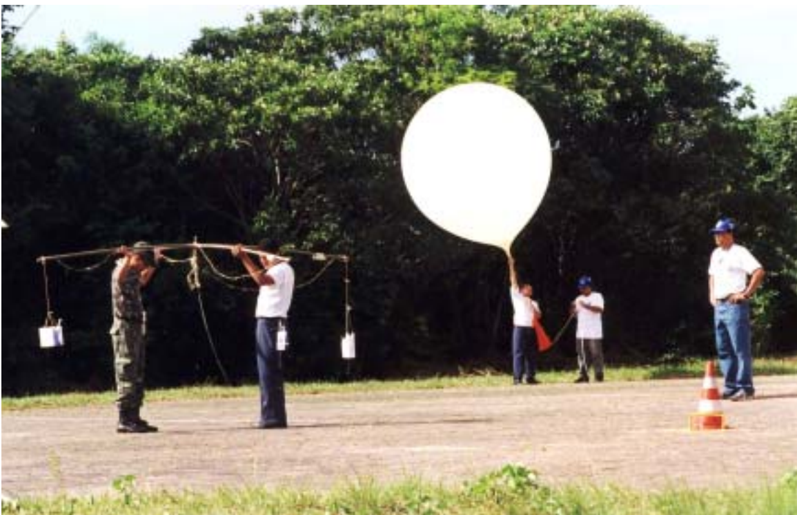
Figure 1. Flight preparation at Alcantara Brazil. The 'rig' is constructed from plastic pipes and is supporting 4 radiosondes.
