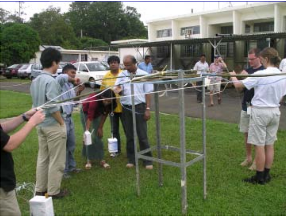
Figure 2. Pre-flight preparations in Mauritius, here the 'rig' is made from bamboo; sourced locally, sustainable and in plentiful supply.
