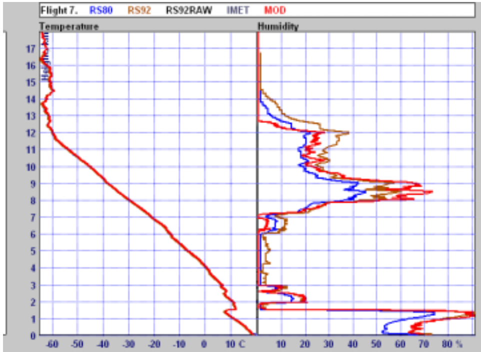
Fig. 3.5 Temperature and relative humidity comparison displayed as a function of height, with results shown from MODEM MKII, Vaisala RS80 and Vaisala RS92
