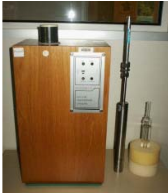
Figure 8 : Cells available in Météo-France, from left to right: gallium, mercury and water cells
