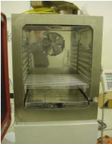
Figure 12. Heraus Votsch 4030 Environmental Chamber (left), split stream chamber (right) .
