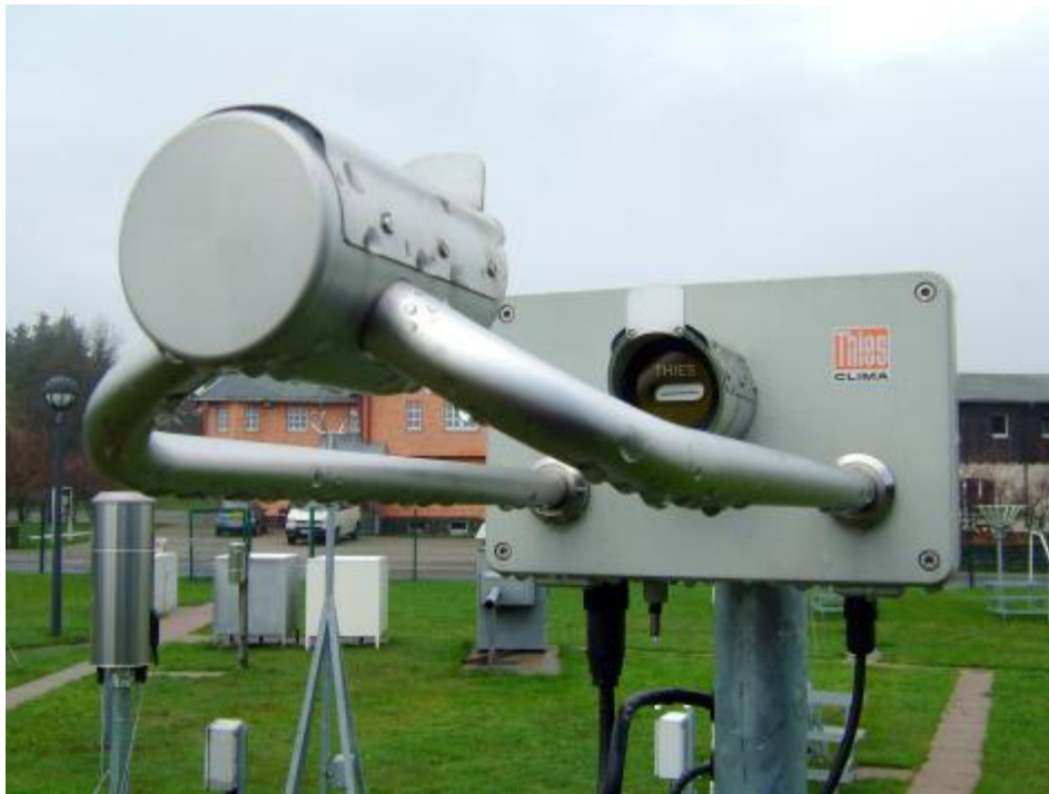
Figure 1: The Laser Precipitation Monitor manufactured by Thies. The square box contains the laser diode and all electronics. The receiver is mounted in a small enclosure opposite to it. In the lower left corner of the picture the Pluvio weighing rain gauge can be seen that served as an intensity reference for this intercomparison.
