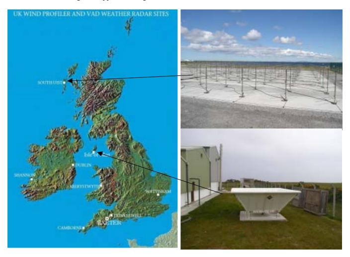
During 2005 the original LAP3000 systems have been upgraded to the new digital signal processing being offered by Vaisala. Whilst replacing a number of redundant units it is expected that the upgrades will offer enhanced remote control & monitoring and improved Quality Control through the improved signal processing options. (i.e. multi-peak, wavelets).
