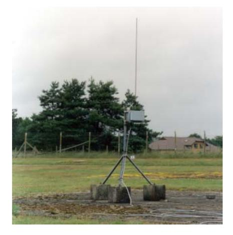
Fig. 2.1 ATD whip antenna used for observations at 10 kHz or 13.6 kHz [frequency can be changed using software]
