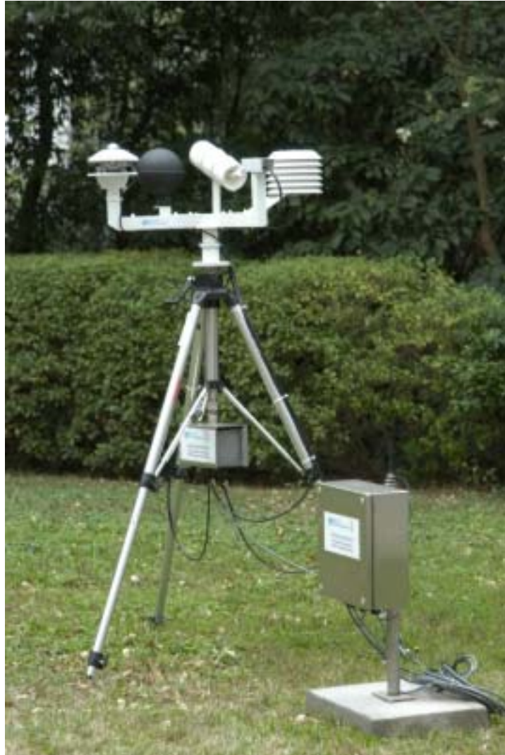
Figure 1: Wet Bulb Globe Temperature (WBGT) equipment developed by the Hong Kong Observatory for heat-stress measurement
