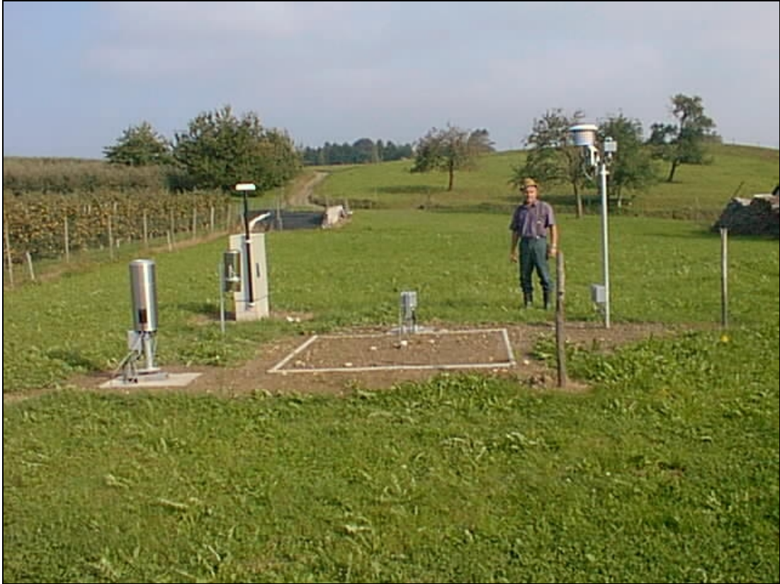
Figure 3: View of the station area, from left: automatic precipitation sensor, Hellmann-sampler, box with AMDA-computer inside and wireless set, area for soil temperature sensors, mast with radiation shield for air temperature and relative humidity sensors and sunshine duration sensor.
