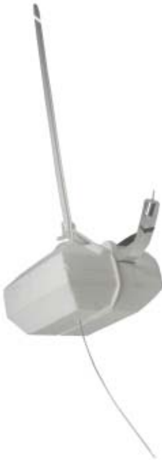
Figure 2.1.4 New Graw DFM-06 radiosonde + temperature mount from previous DFM-97 radiosonde
