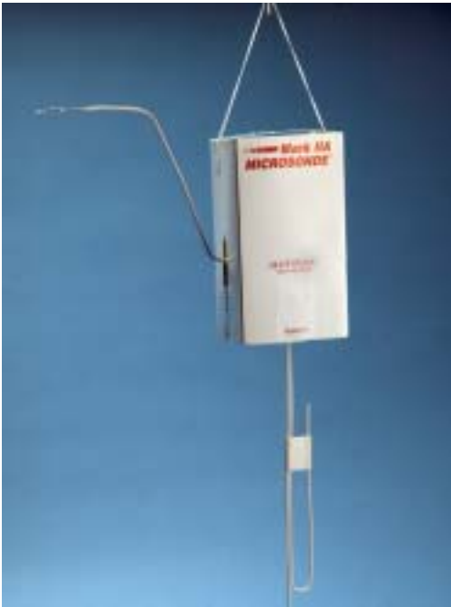
Figure 2.1.6 Lockheed Martin Sippican radiosondes, MKIIa as used in Brazil intercomparison, LMS-6 designed following the WMO high quality Radiosonde Intercomparison in Mauritius
