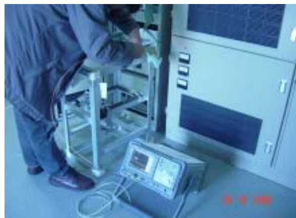
Figure 6: Spectrum Analyser and a Measurement with it.
