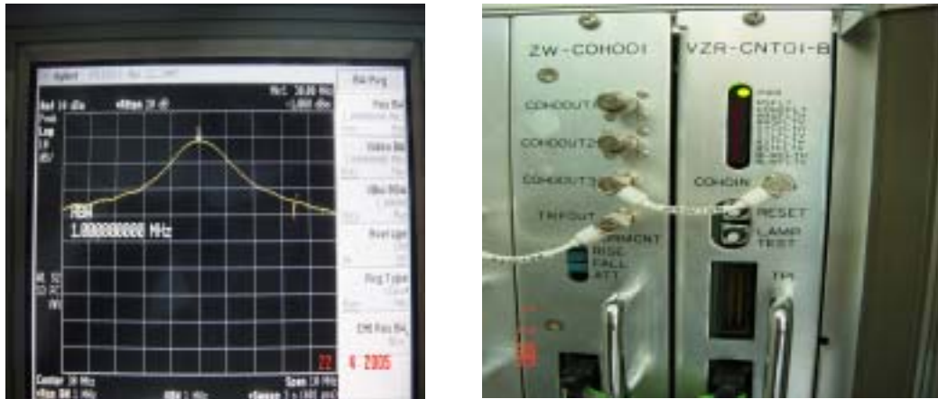
Figure 33: TX IF Out Measurement.
