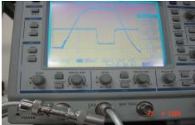
Figure 20: TX Klystron Pulse and Current from Test Point at TX Front Panel.
