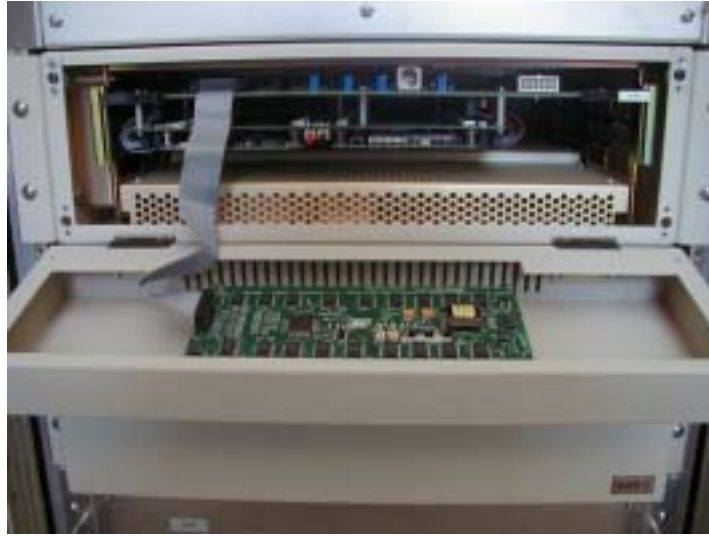
Figure 57: A Radar Control Processor.
