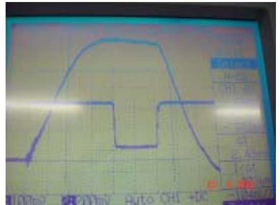
Figure 20: TX Klystron Pulse and Current from Test Point at TX Front Panel.
