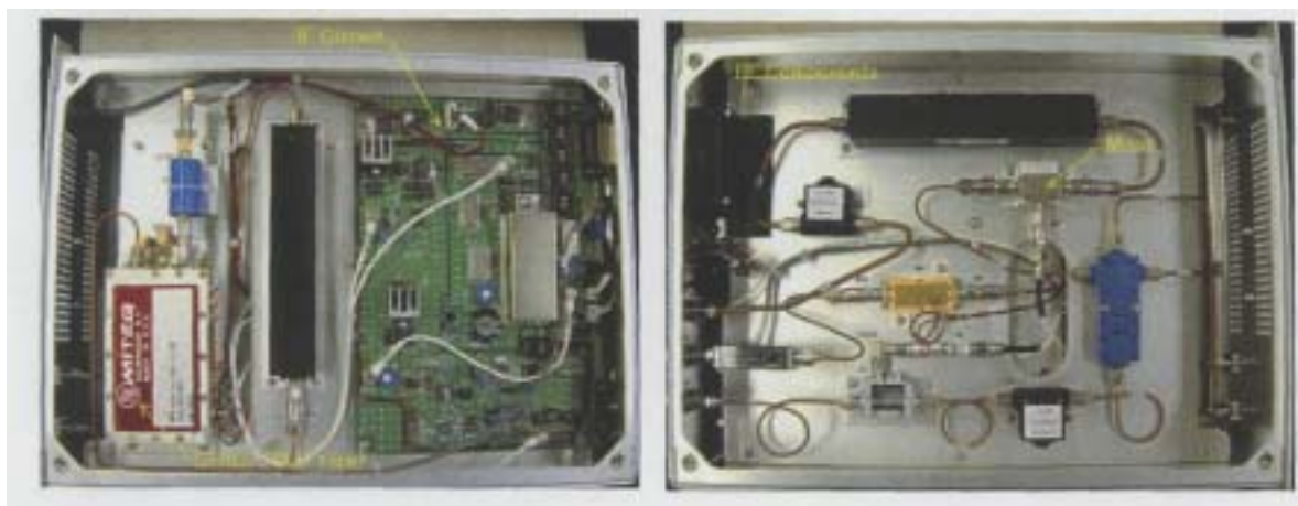
Figure 14: Inside of Receiver Hardware (IF and RF Sections)
