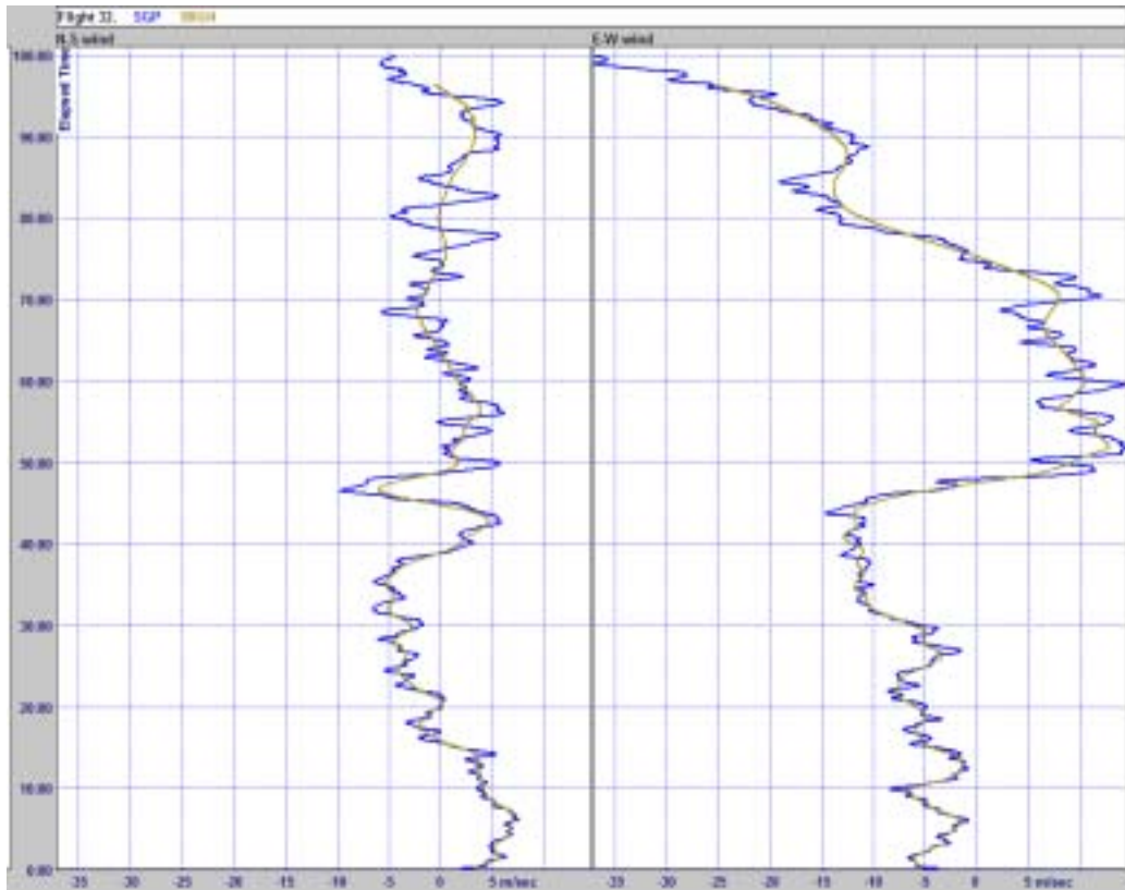
Fig.6 Simultaneous measurements of wind from Vaisala (SGP) and IMS (MKII4) from flight 32 on 28.10.04
