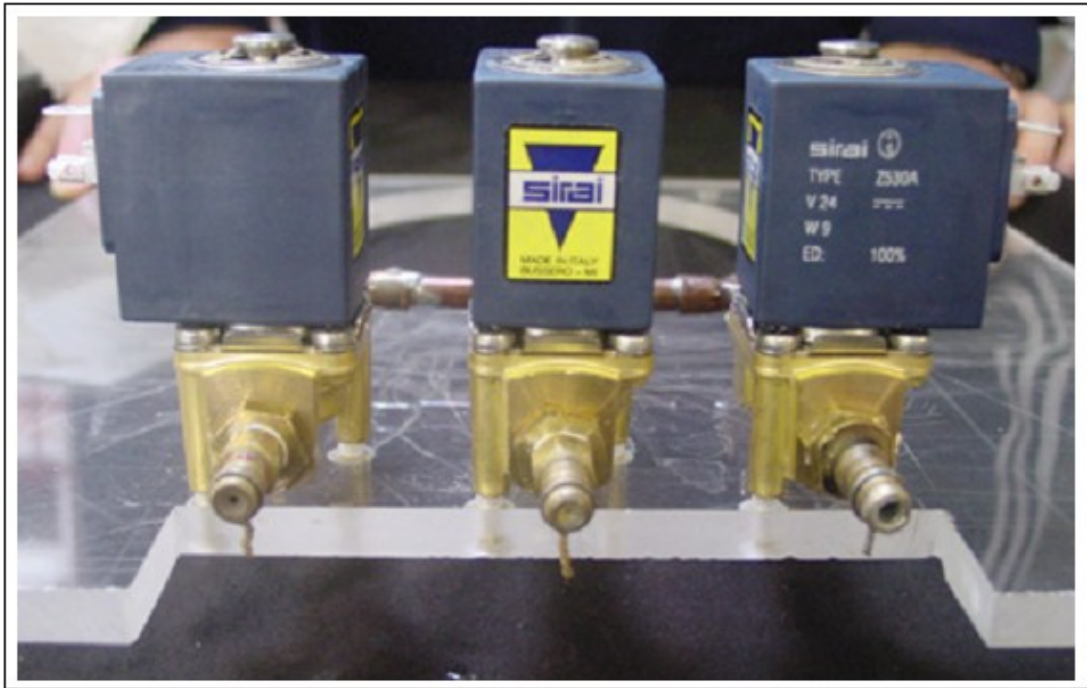
Figure 3: The three electrovalves that allow to combine different nozzles diameters in order to produce a wide range of water flow rates.
