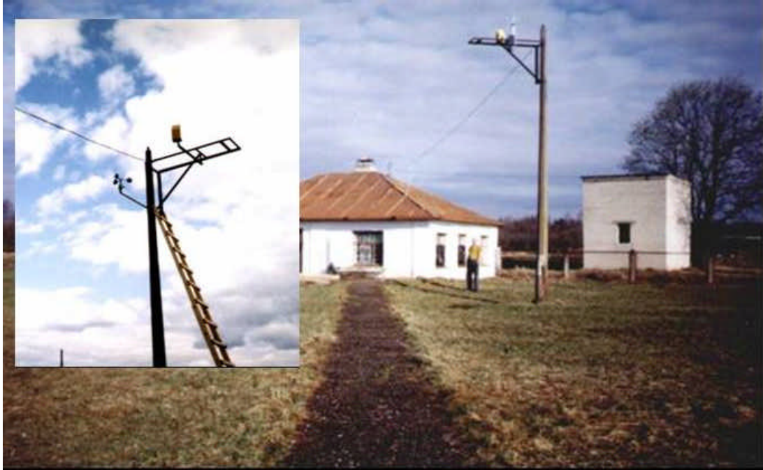
Figure 3. Comparisons of LSR –11 with the Russian Federation State Standard of Rain Precipitation on the experimental site of State Hydrological Institute. Valday, Novgorod Reg. May-September 2004.
