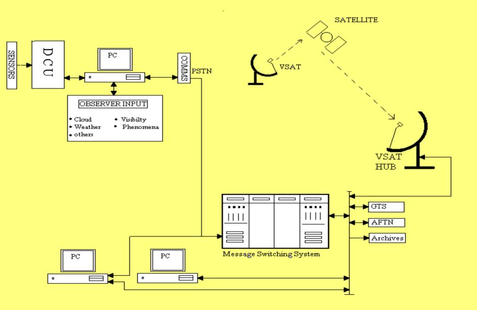
◆ The Observer console is a user friendly system that displays meteorological information coming from a Data Collection Unit (DCU) as well as allow an observer to manually supplement other meteorological variables such as cloud, visibility, weather, phenomena, etc. into the overall station observation process. The console automatically accepts data from a DCU and log this information in its local database.
