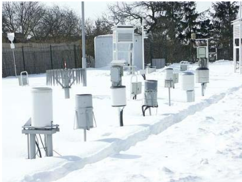
Figure 1. The experimental polygon of precipitation gauges at the Bratislava-Koliba meteorological station.
