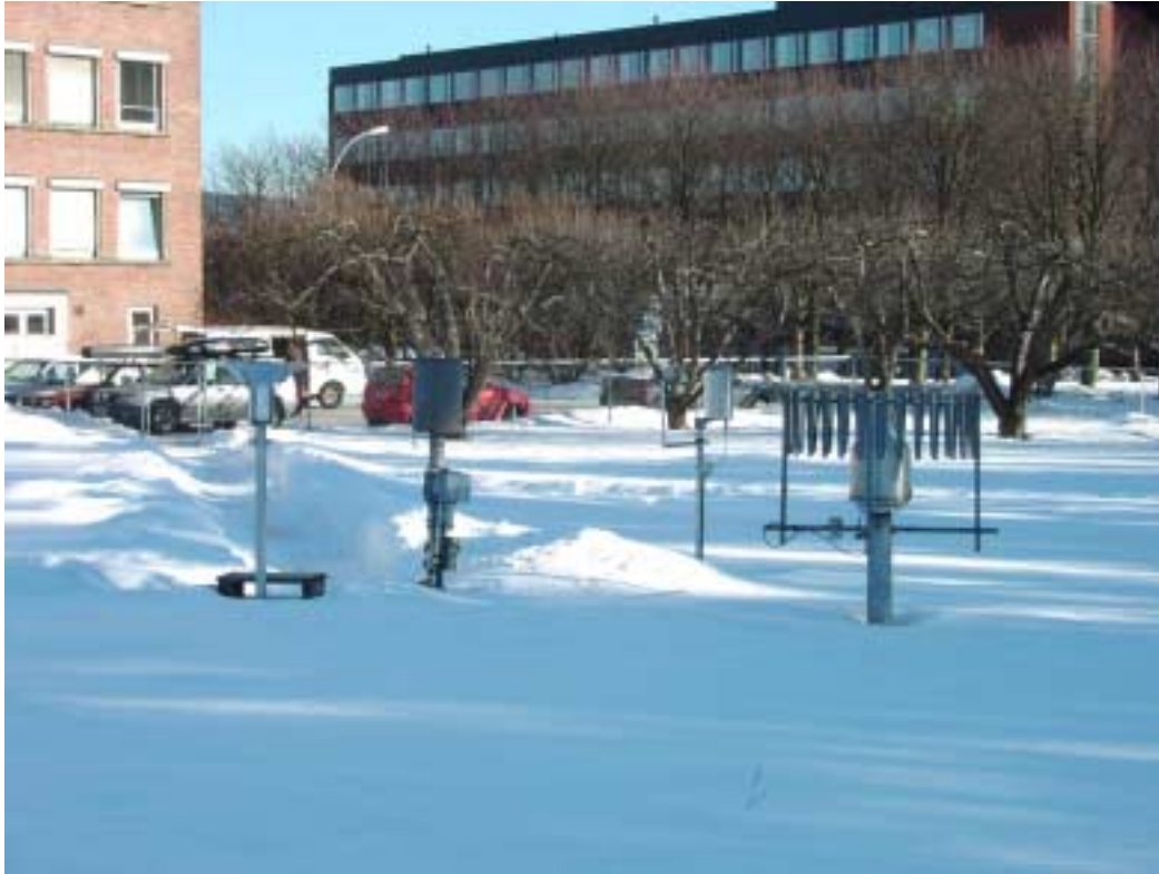
Figure 1: Picture showing the manual (to the left) and the automatic (to the right) precipitation gauges.
