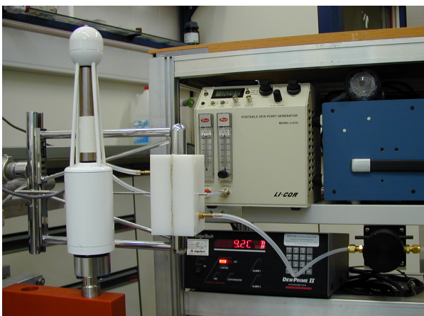
Figure 3: Calibration facility for open path hygrometers
