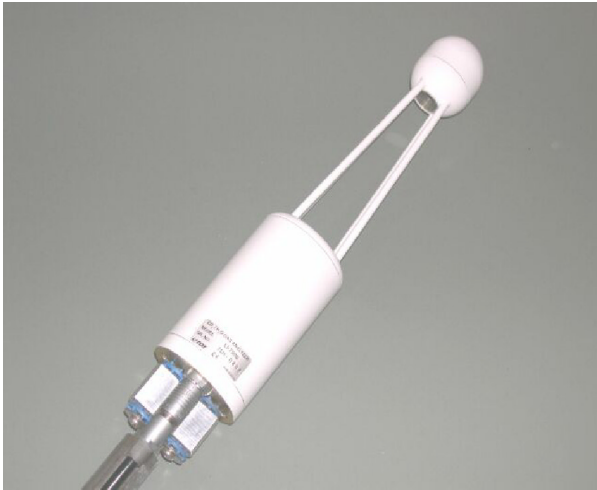
Figure 1: LI-7500 sensor head
