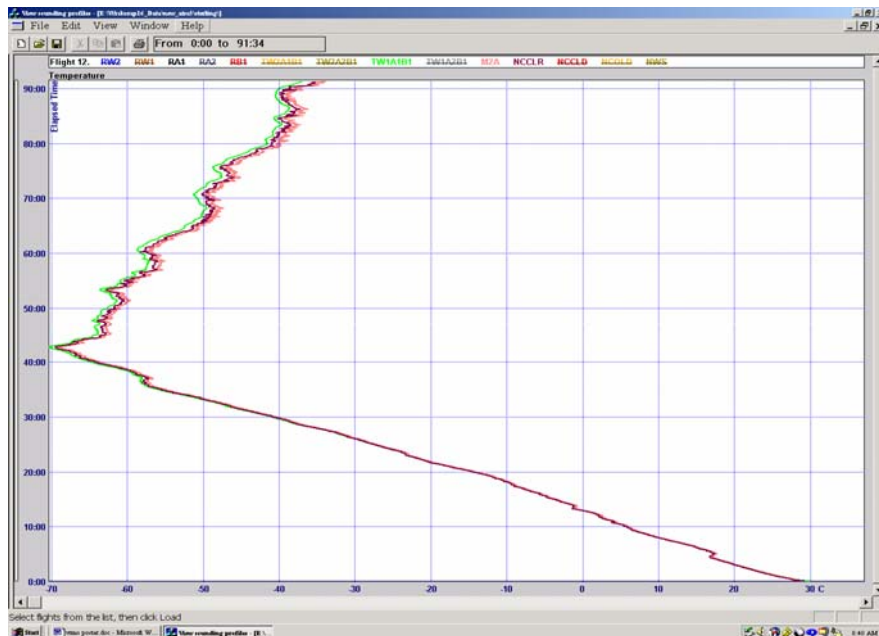
Figure 3. Illustrates comparison between ATM temperature (green line) and uncorrected chip temperature (light red line) and corrected chip temperature (dark red line). The correction applied to the chip thermistor is in the proper direction, but in this example the amount of the correction is not considered to be large enough.
