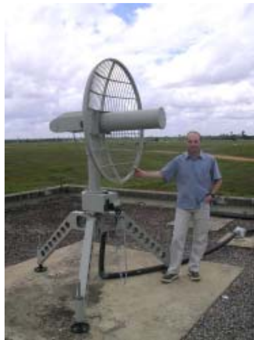
Fig.2 Sippican MKII Radiosonde and Internet IMS 1500 radiotheodolite.
