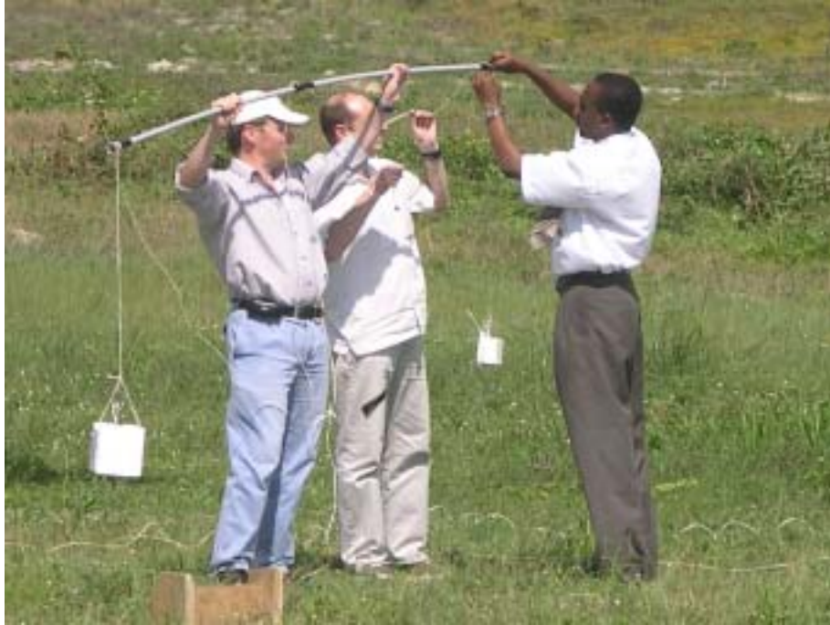
Fig.3 Preparing to launch a Sippican / Vaisala RS92 twin flight, Dar-es-Salaam.
