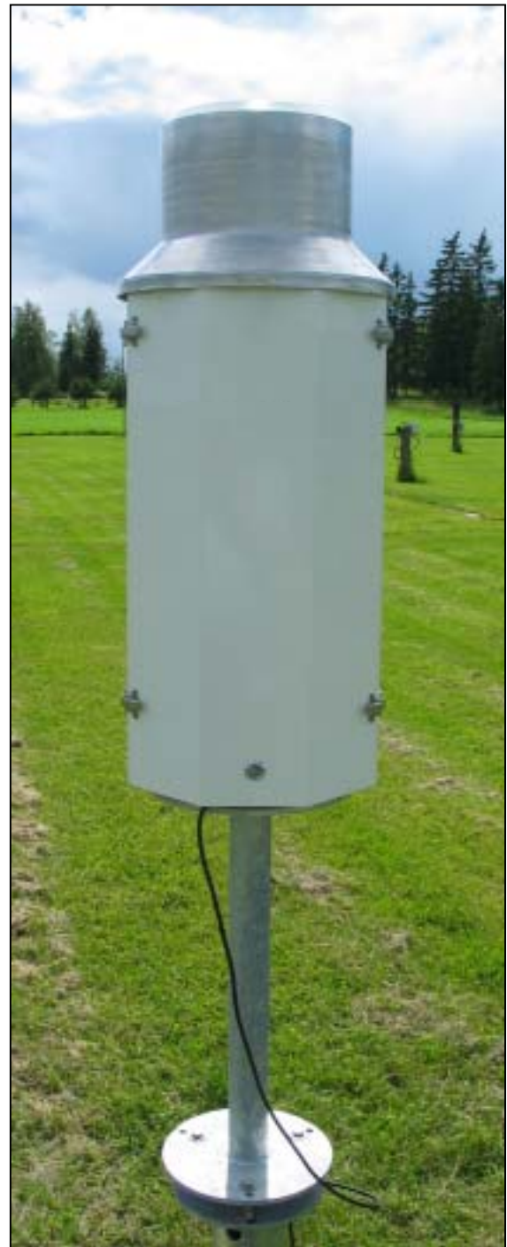
to 150 % in a single rainfall, being highest in slight rains. Fig. 6. The Vaisala gauge installed on the FMI Jokioinen test field.
