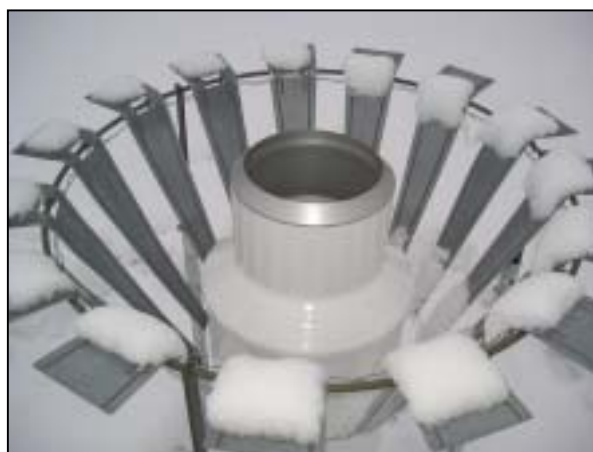
Fig. 7. The gauge on the Vaisala test field with wind shield.
