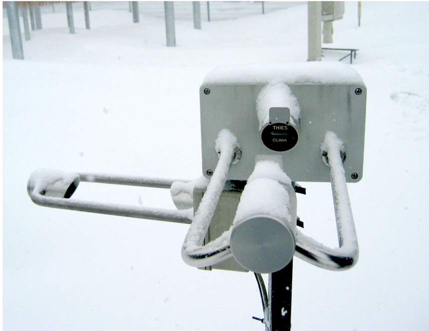
Figure 2. The two Thies disdrometers at Wasserkuppe.
