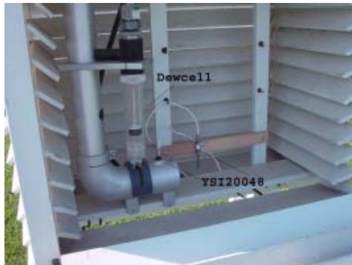
Figure 3 - Field reference temperature sensor (YSI20048) in aspirated wooden screen.
