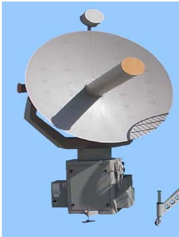
Figure 5. IMS 2000 Radiosonde Ground Receiver
