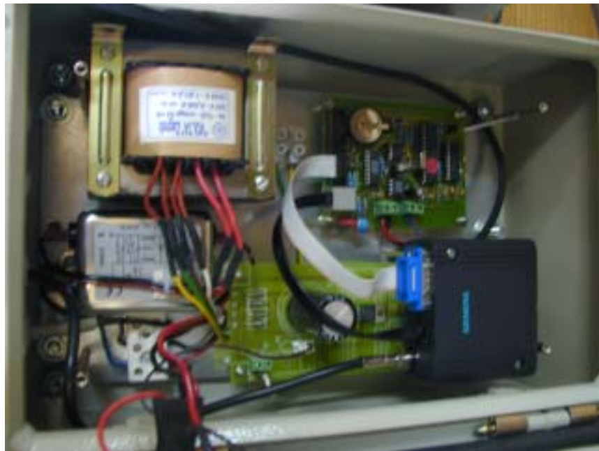
Figure 2. Processor module and data logger, type a-ombro ( Tritonel Multimedia, Croatia )
