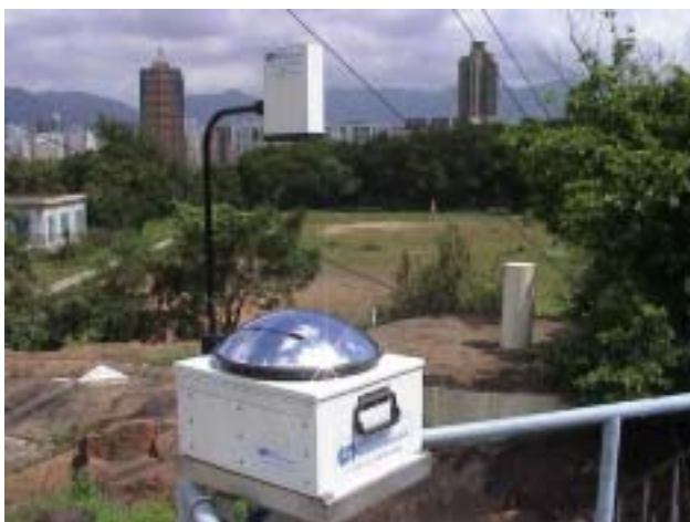
Figure 2(a): The total sky imager takes snapshot of the reflected sky from a convex mirror every 10 minutes. The snapshot is useful for observing clouds and assessing cloudiness during daytime.
