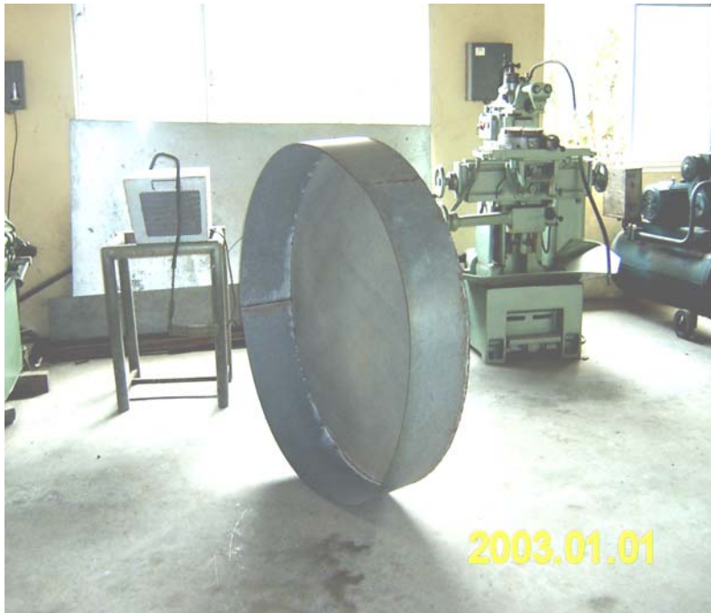
Fig.10.0 Class A Pan Evaporimeter under construction
