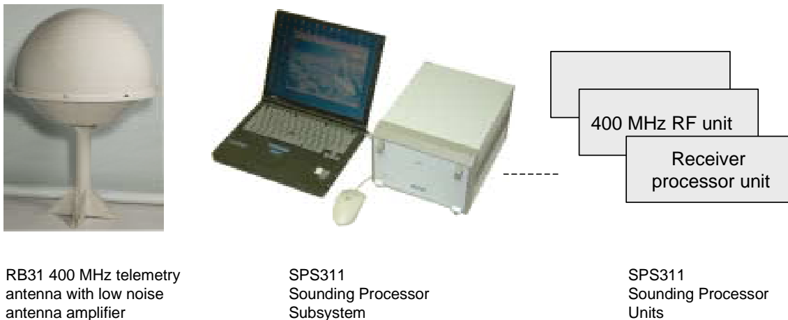
Figure 1. The Vaisala Sounding Processing Subsystem SPS311 with Software Defined Radio
