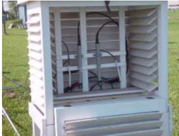
Figure 1 - Test sensors in non-aspirated Stevenson screen.
