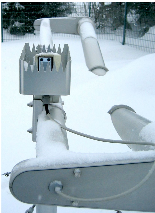
Figure 3. The Vaisala FD12P Present Weather Sensor at Wasserkuppe.
