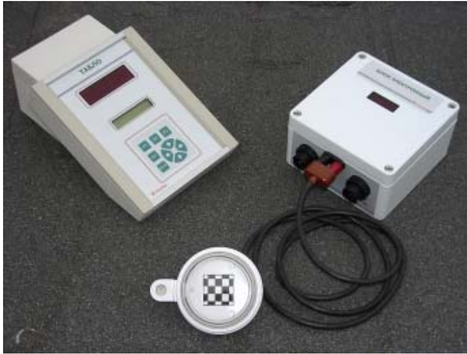
Figure 1. Pyranometer with unit and information board. External View.
