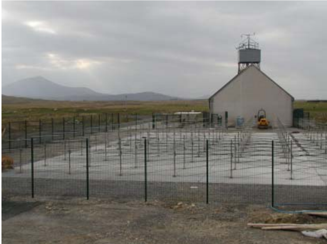
Fig.4 Operational wind profiler observing at 64 MHz on the island of South Uist.
