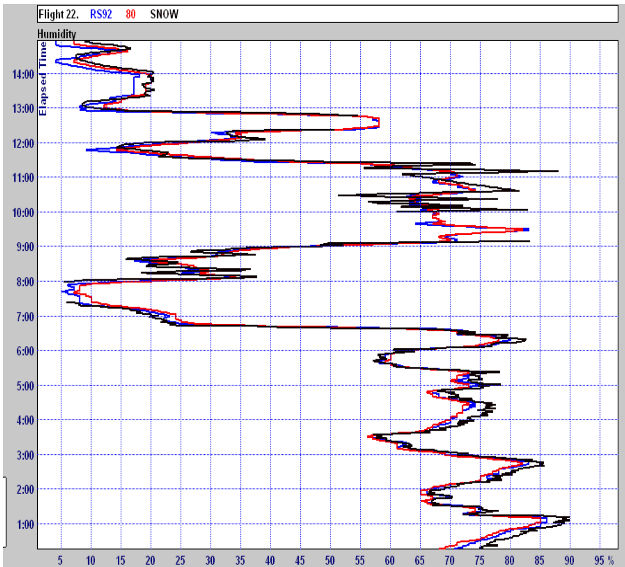
Figure 4(a), Simultaneous relative humidity measurements of RS92 (blue), RS80 (red) and Snow White (black). The Y axis is time from 0 to 15 minutes and the X axis is relative humidity (%)
